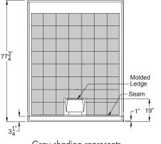
Gray shading represents plywood reinforced walls
